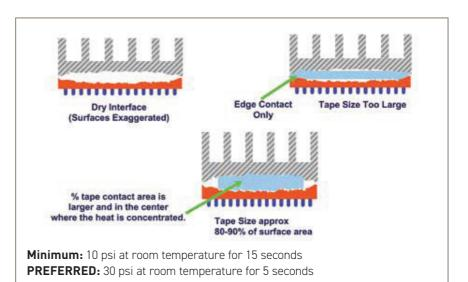
Note that typically 70% of the ultimate adhesive bond strength is achieved with initial application, and 80-90% is reached within 15 minutes. Ultimate adhesive strength is achieved within 36 hours; however the next manufacturing step can typically occur immediately following the initial application.
